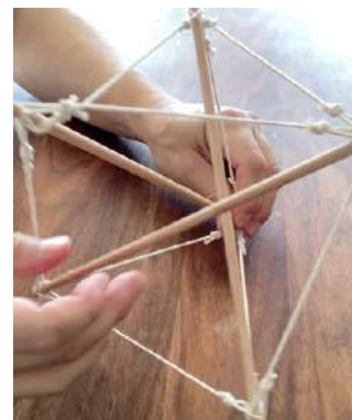
Fig. 12. After connecting all tendons, the state of tensegrity occurs.
